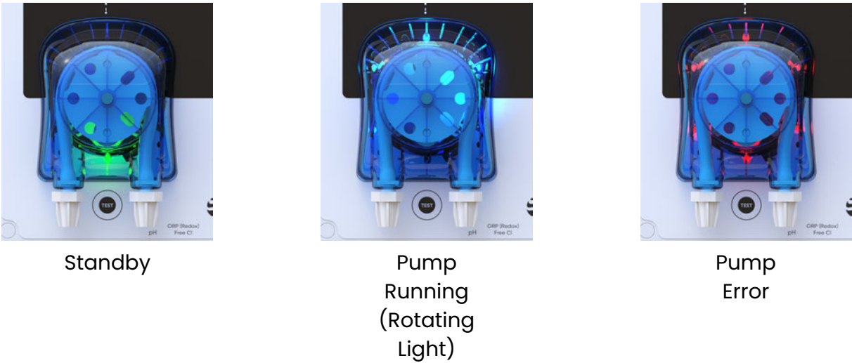
Fig. 4 Meaning of the Dosing Pump Indicator LEDs
