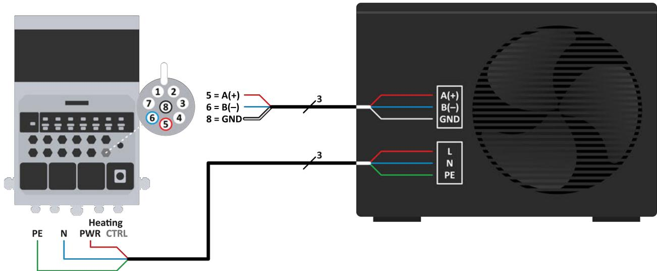
The control cable between the main control unit and the heat pump must be laid separately from any power cable in a separate cable conduit or cable tray.
