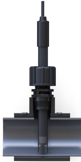
To reduce the risk of damage to the electrodes from solid particles in the water flow, we recommend installing the electrode tip outside the main water flow, approximately 5-10 mm from the bottom of the pipe.
