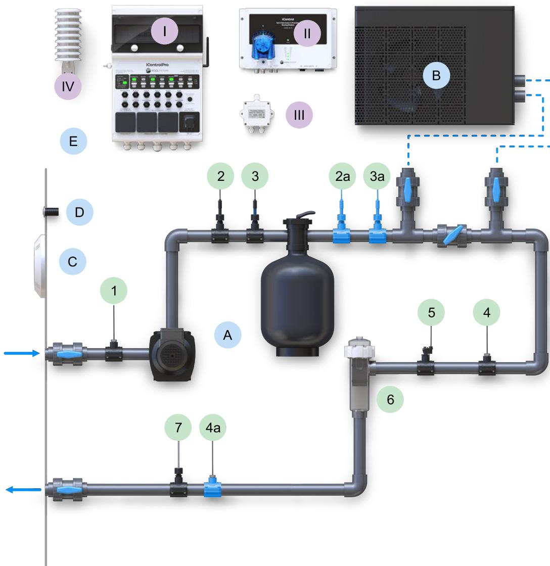
Fig. 2 Saltwater Pool Installation with Bypass for the Electrolytic Cell. The Water Flow Sensor Must be Installed in the Bypass.
