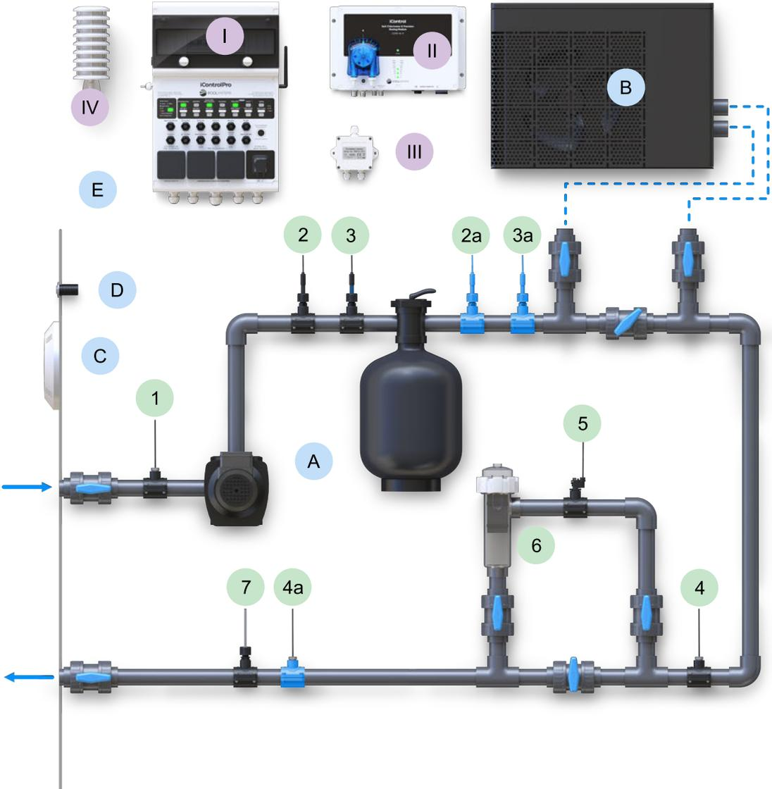
Fig. 3 Alternative Mounting Position of the Electrolytic Cell
