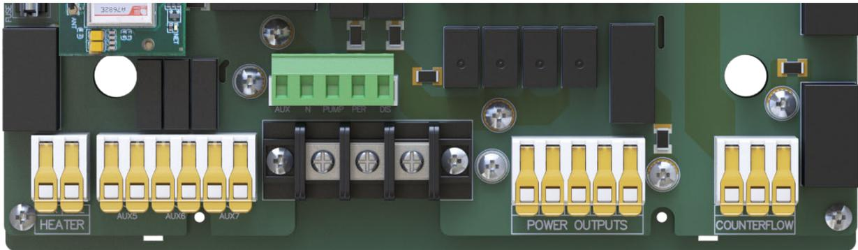
Fig. 22 Internal Connection Points for Pool Technology and Mains Power – 1-phase version: SDWM002-PS(D)114122
